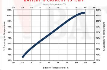
batteries at low temperature or going into thermal runaway at high temperature.
